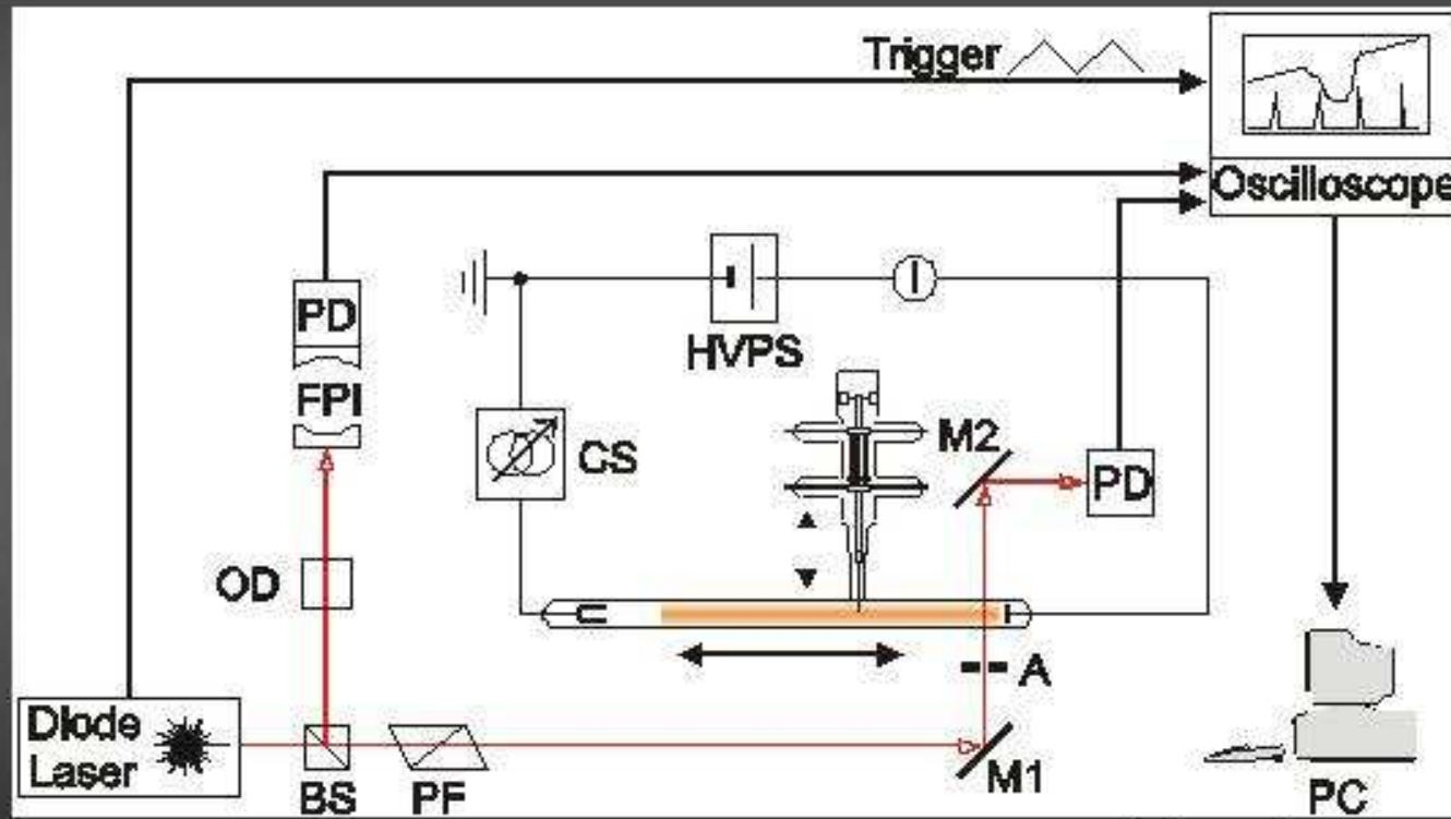
BS Beam Splitter, CS Current Source, HVPS High Voltage
